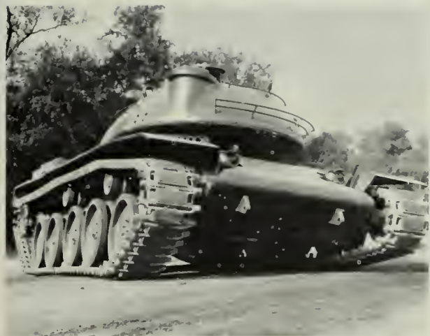
HYDRO-PNEUMATIC suspension system for tanks, developed by Army, will enable them to change ground clearance.
